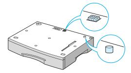
3 Align the machine with the optional tray and lower it into place on the tabs and connector.
